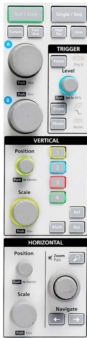
Efficient and intuitive front panel provides critical controls while still leaving room for the massive 15.6" high definition display.
